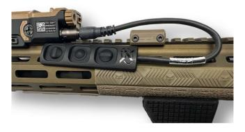
NOTE: On the inline version there is a screw that is longer than the other. Make sure you use the long screw on the side where the removable tab is located.
